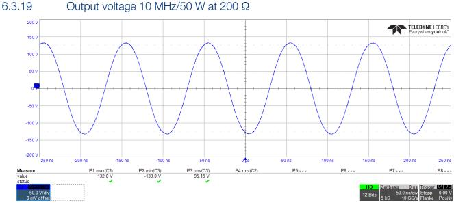
Output voltage 10 MHz/50 W at 200  $\Omega$
