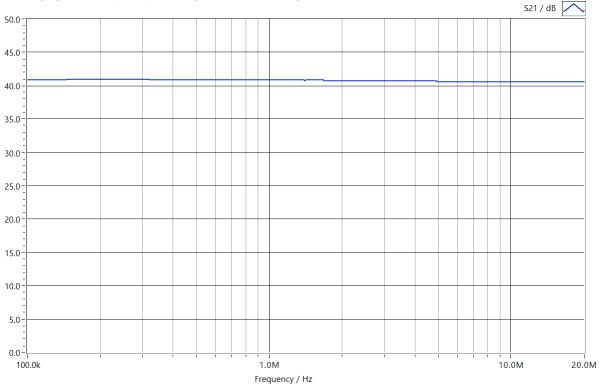
6.1.2 Output voltage 100 kHz/50 W at 50  $\Omega$
