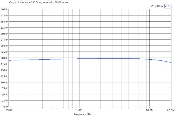
Network Analyser HP8751A (S.-No.: 3315J01756), Test Set 87512A (S.-No. MY43100614) Bidirectional Matching Transformer B-MT-1 Output impedance 200 Ohm, input with 50 Ohm load
