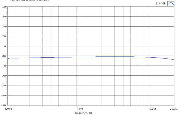
Network Analyser HP8751A (S.-No.: 3315J01756), Test Set 87512A (S.-No. MY43100614) Bidirectional Matching Transformer B-MT-1 Insertion loss 50 Ohm to 200 Ohm
