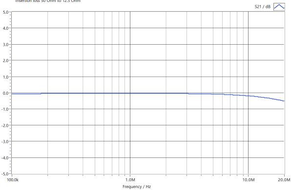
Network Analyser HP8751A (S.-No.: 3315J01756), Test Set 87512A (S.-No. MY43100614) Bidirectional Matching Transformer B-MT-1 Insertion loss 50 Ohm to 12.5 Ohm
